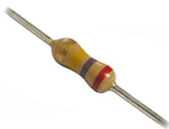
Function: **Indicates the tolerance band of the resistor (+/- 5%) etc.**
