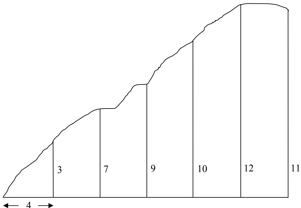
Offsets of lengths 3, 7, 9, 10, 12 and 11 metres are measured at intervals of 4 m as shown.
