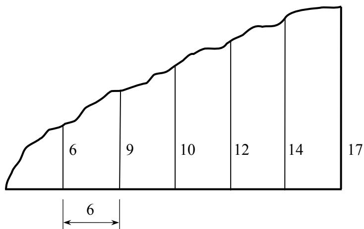
Offsets of lengths 6, 9, 10, 12, 14 and 17 metres are measured at intervals of 6 metres as shown.
