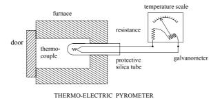
Applications for both would be measuring temperature in heat treatment furnaces. (one description + application) 7 + 1
