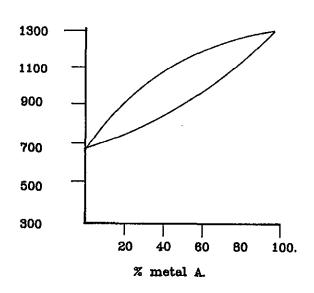
(c) With reference to the diagram on the right hand side above, determine for a 40% metal A, the ratio of the phases at 900°.
