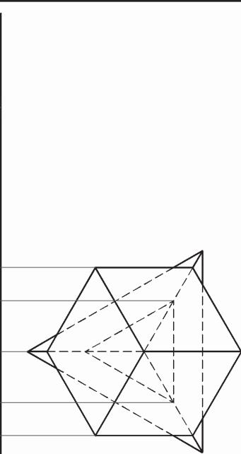
**A-3.** The image below shows a sign outside the offices of a company called 'Key Technologies'. In the sign, a truncated copper pyramid is intersected by a triangular steel prism. The drawing on the right below shows the elevation and incomplete plan of the solids which penetrate each other.
