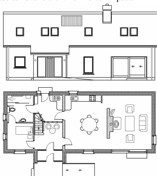
7. A new house with an internal width of 7.0 metres, has a traditional cut roof which is slated and has a pitch of 45 degrees, as shown in the accompanying sketch. The roof is designed to incorporate bedroom accommodation in the attic space.
