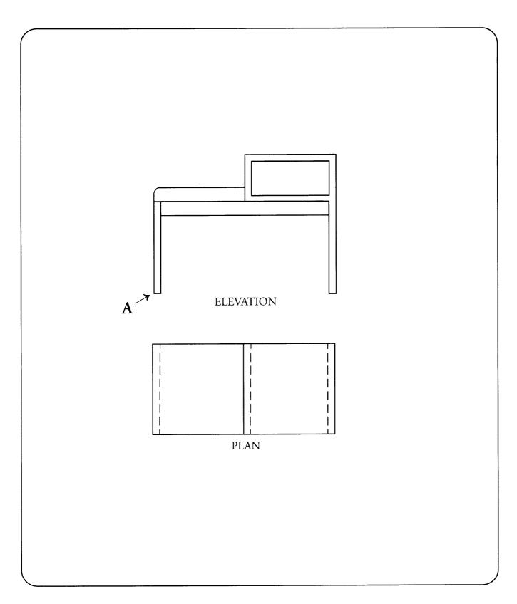
(a) Draw in proportion an isometric view of the table/seat on the isometric grid on the next page. The position of corner A is given.
