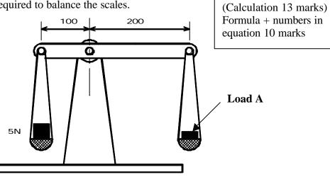
Calculation  $\underline{100 \times 5N} = \underline{200N} \times A$
