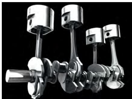
The **pistons** in an engine:
