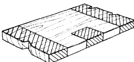
Meaning: 4 marks - indicated material to be cut away, waste material.
