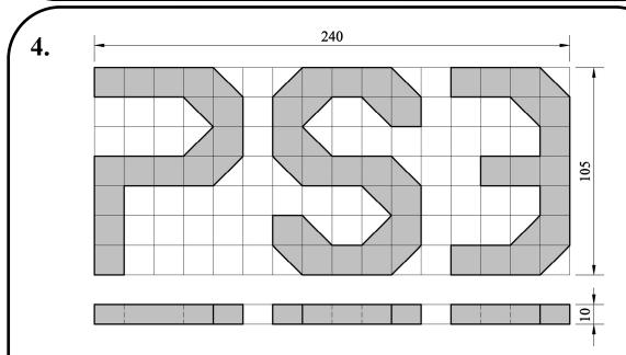
The figure shows the elevation and plan of a logo for a **games console - PS3**. The grid in elevation is made up of 15mm squares and the thickness in plan is 10mm.
