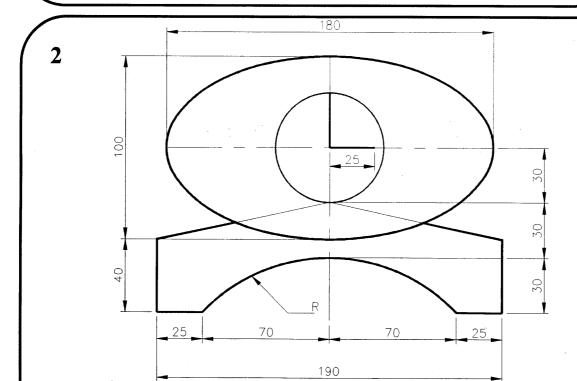
The figure shows the design of a **CLOCK** containing an ellipse, with Major and Minor Axes 180 and 100 respectively.
