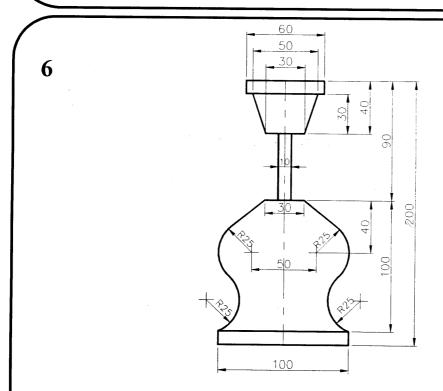
A design for a **CEILING LIGHT** is shown. Draw the given design, showing clearly all constructions and points of contact.
