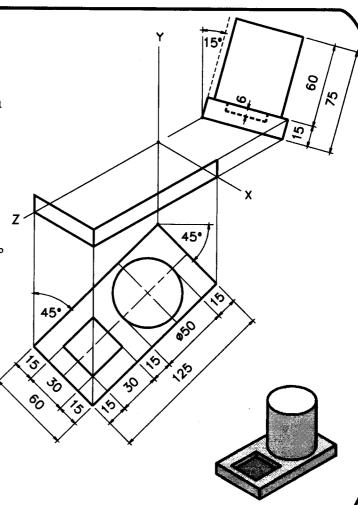
4. The figure shows the elevation and plan of a closed container.
