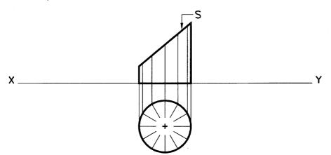
**11.** The elevation and plan of a ring are shown. Draw a <u>freehand</u> pictorial sketch of the ring in the space provided.
