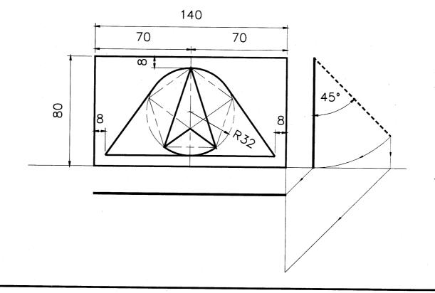
3. The figure shows the incomplete isometric projection of a paper weight using the axonometric axes method. The side elevation and plan are also shown in their required positions.
