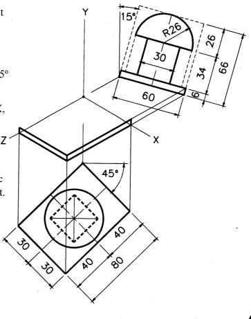
**4.** The elevation, plan and end view of a laptop writing unit are shown.
