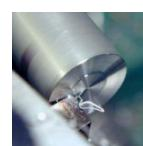
**Parallel turning** is the creation of cylinders by moving the tool parallel to the work on the lathe.
