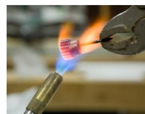
(ii) Hardening – a piece of high carbon steel is heated to a cherry red. It is then quenched rapidly in water or oil to make the steel hard. The hard steel will also be brittle and may need to be tempered to make it suitable for use.
