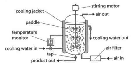
(i) Explain the function of the temperature monitor and cooling jacket.
