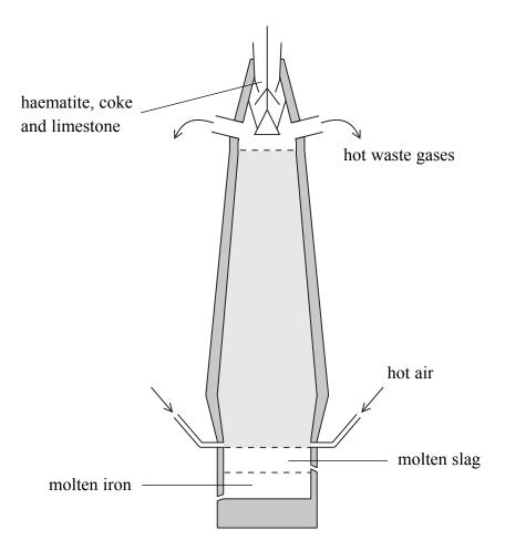
(a) (i) During this extraction process, coke (a form of carbon) burns. The reaction is exothermic.
