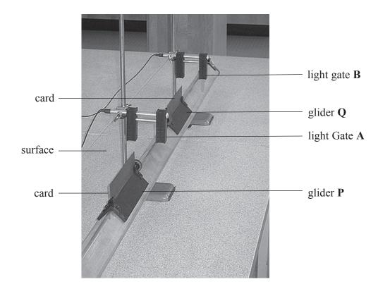
The mass of glider P is 2.4 kg. This glider is moving toward Q at a constant velocity of 0.6 m/s. Glider Q is stationary.
