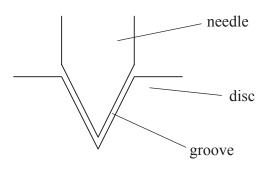
The shape of the groove determines the amplitude and frequency of the movement of the needle.
