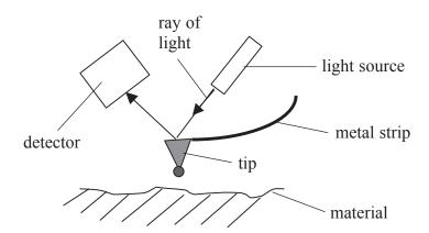
The bottom of the tip is negatively charged. It is attracted or repelled by the charge on the surface of the material.
