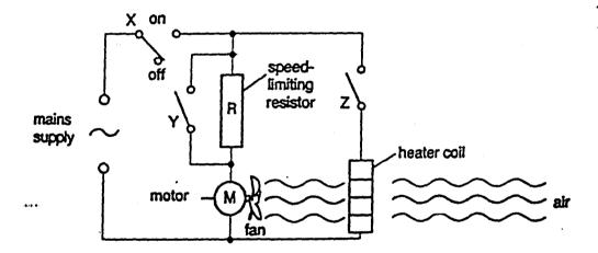
Which switches should be closed so that the motor runs at high speed and the heater blows hot air?
