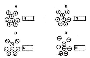
25 Different metals are separated by passing them under an electromagnet, which attracts and lifts out some of the metals.
