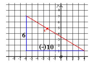
The figure shows a representation of this vector. Forming the right-angled triangle we have the length of the two shorter sides. Using Pythagoras we can determine the length of **c** as follows:
