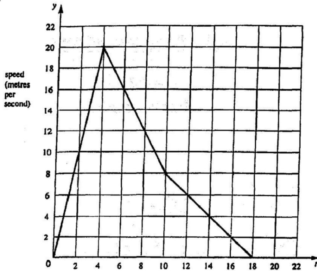
(b) Deceleration  $d = \frac{\text{Change in speed}}{\text{Time}} = \frac{8}{8} = 1$
