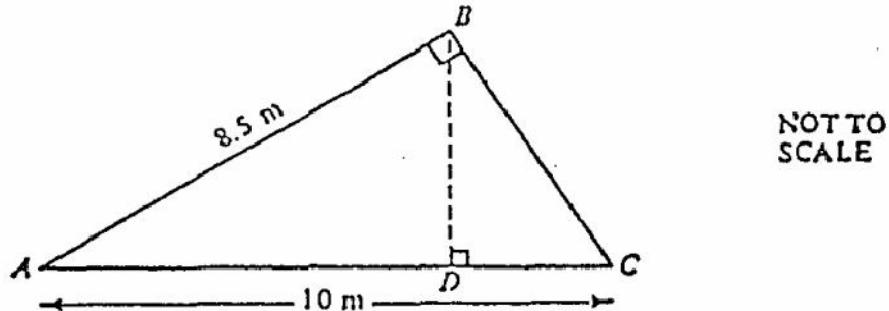
The diagram above shows the cross-section of a factory roof. Given that  $AB = 8.5$  metres,  $AC = 10$  metres and angle  $ABC = \text{angle } BDC = 90^\circ$ , calculate
