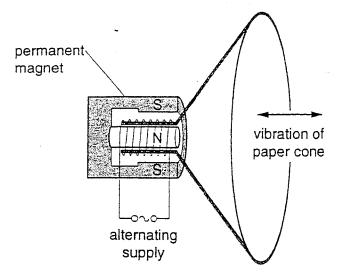
(c) Explain why the cone vibrates when an alternating current passes through the coil.
