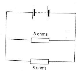
Calculate the combined resistance of the two resistors as shown in the circuit.
