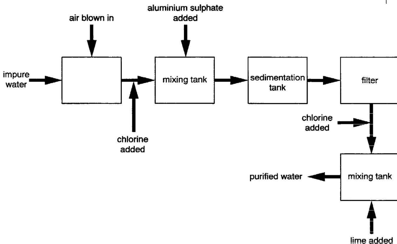
**(d)** Air is blown into impure water to help remove dissolved iron compounds.
