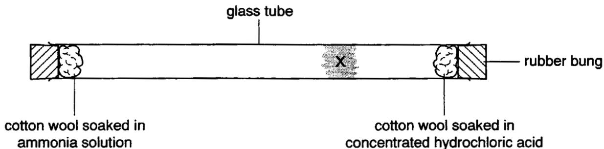
After two minutes, a white solid was seen at point X, where fumes of hydrogen chloride and ammonia had reacted.
