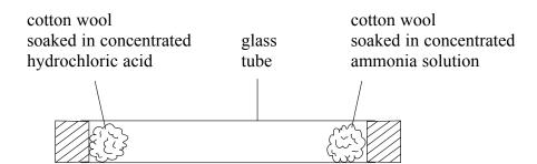
After a few minutes a white solid forms inside the tube. The solid forms when ammonia gas reacts with hydrogen chloride gas.
