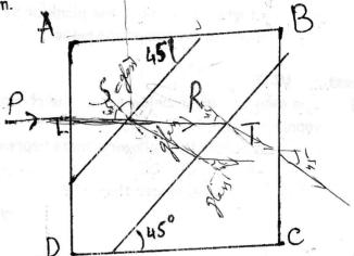
P is the ray of light perpendicular to AD entering the glass cube. Draw the path of P till it comes out of ABCD when ;
