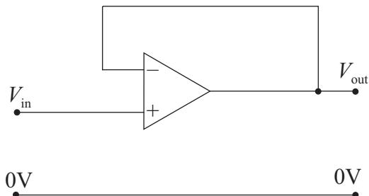
Explain, in terms of the properties of an op-amp, why the gain of this non-inverting amplifier is equal to 1. [3]
