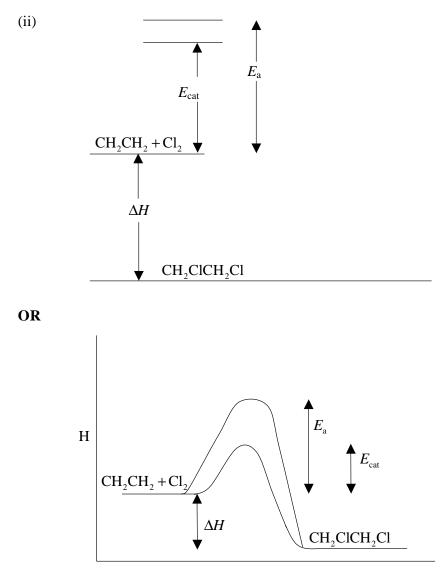
reactants line higher than product line (labels not needed);  $\Delta H$  label;  $E_{a}$  label;  $E_{cat}$  label;
