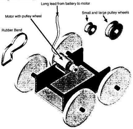
A pupil has made a small battery powered model car. An elastic band will transmit the power from the pulley wheel on the motor, to a pulley wheel on the axle of the model.
