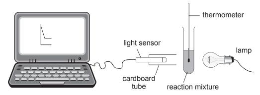
$5\,\mathrm{cm^3}$  of dilute hydrochloric acid was added separately to  $10\,\mathrm{cm^3}$  sodium thiosulfate solutions at four different temperatures. All other factors were kept the same. The results are shown on the grid below.
