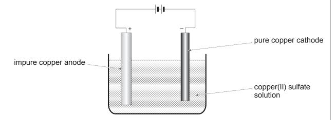
(a) During the process copper(II) ions move to the cathode where they become copper atoms.
