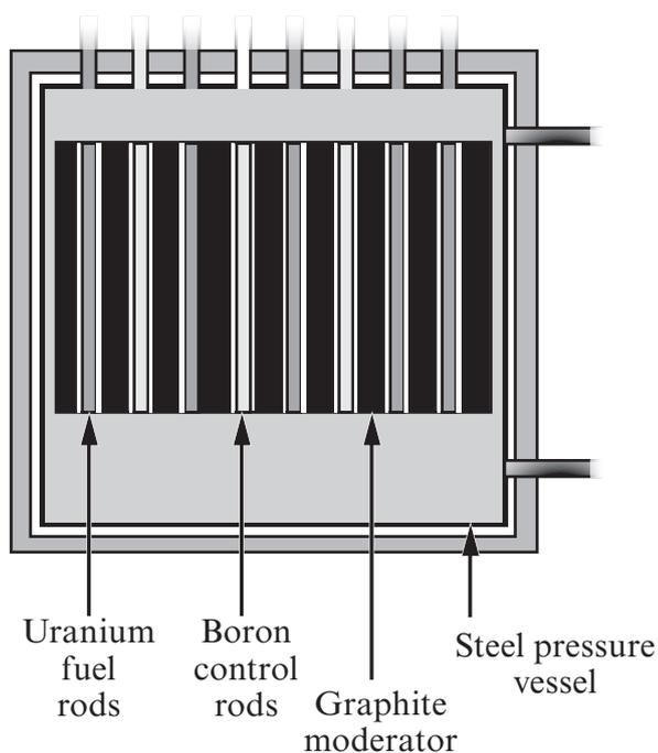
(a) (i) State which labelled part of the reactor slows down neutrons. [1]
