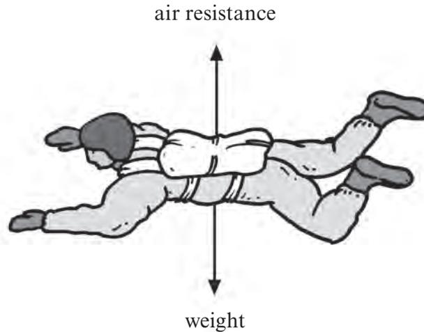
As the skydiver jumps from an aeroplane and falls, his motion will depend on the two forces shown in the diagram.
