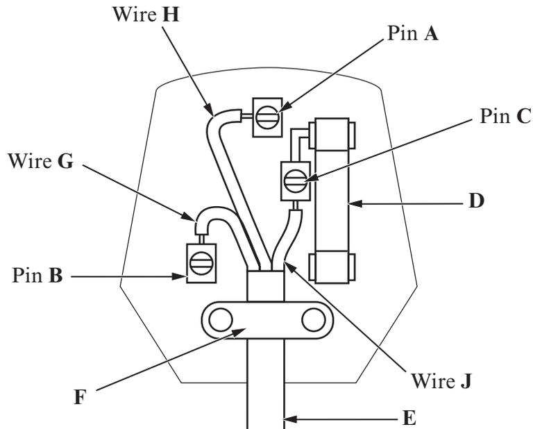
The diagram shows the inside of an electric plug.
