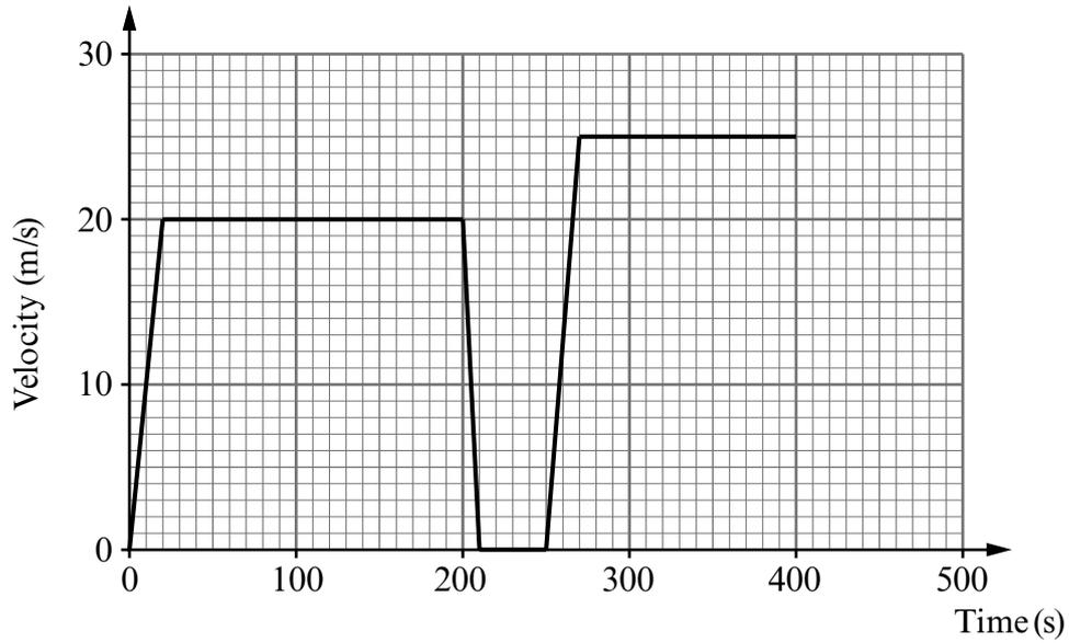
(a) (i) Using information from page 2, calculate the initial acceleration of the train. [2]
