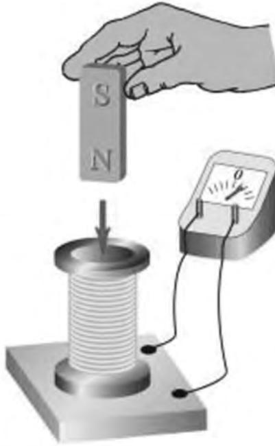
When the North Pole of the magnet is pushed into the coil, the meter needle flicks to the right and returns to the middle.
