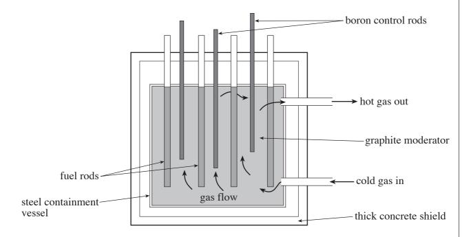
In the reactor, energy is released by fission and is the result of a controlled chain reaction.
