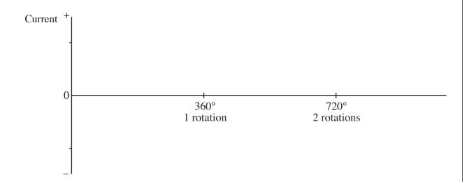
(iii) Increasing the speed of rotation of the coil increases the size of the output current and voltage. State one other effect increasing the speed of rotation has on the output from the generator. [1]
