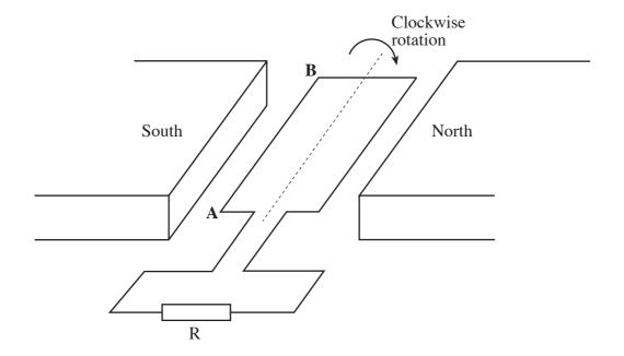
As the coil rotates, an alternating voltage is produced which drives an alternating current through the coil and resistor R.
