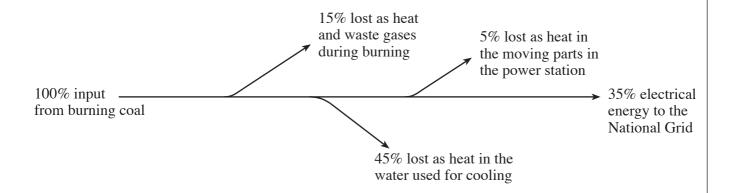
This power station is 35% efficient in generating electricity. It releases 65% of the energy from burning coal into the environment,
