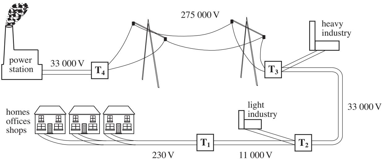
**T<sub>1</sub>, T<sub>2</sub>, T<sub>3</sub> and T<sub>4</sub>** are sub-stations which use transformers to ‘step up’ or ‘step down’ the alternating voltage.
