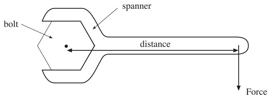
A force at the end of the spanner produces a **moment** about the bolt.
