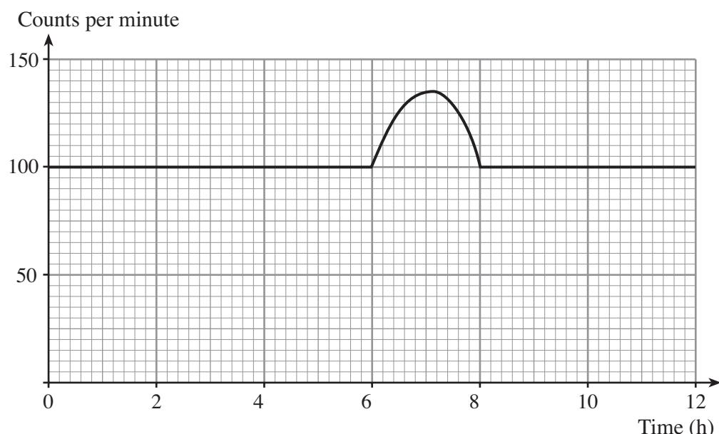
The graph shows the readings produced on the detector over a period of 12 hours when producing a batch of foil.
