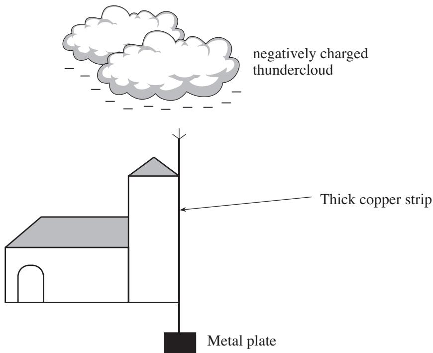
The negative thundercloud causes a movement of charge in the lightning conductor. Positive and negative ions are produced in the air around the sharp points. The movement of these ions reduces the build up of charge on the cloud making a lightning strike less likely.
