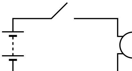
**Each time that he presses the switch, the buzzer makes a sound.**
