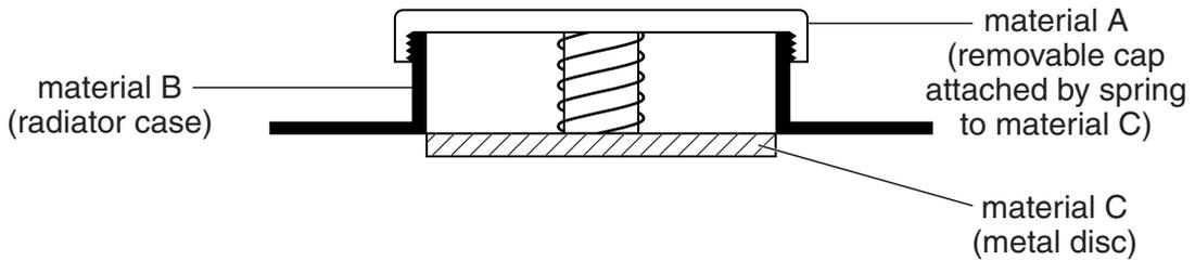
Explain the properties required of materials A, B and C to prevent the cap being removed when the radiator is hot but to allow it to be removed when the radiator cools.
