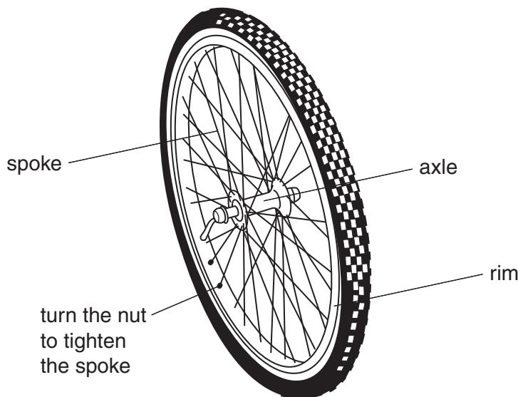
He clamps the axle firmly and uses a force to make the rim bend (deflect) sideways.
