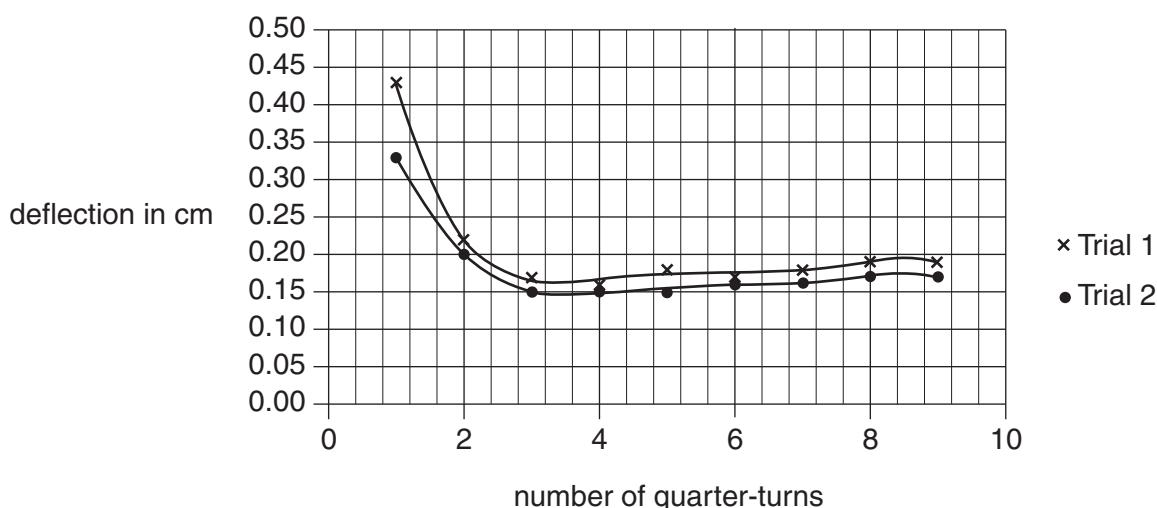
The graph shows that the wheel is flexible if the spokes are loose and stiff if the spokes are tight.
