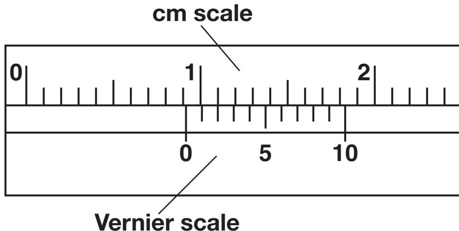
Use the Vernier scale to determine the diameter of the button.
