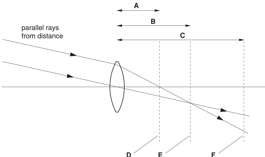
This ray diagram shows how a lens produces an image of the top of a distant object.
