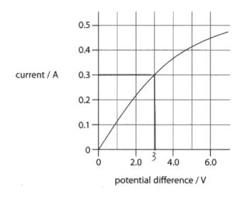
Calculate the resistance of the lamp when the current in the lamp is 0.3 A.
