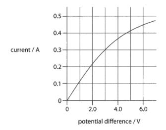
Calculate the resistance of the lamp when the current in the lamp is 0.3 A.
