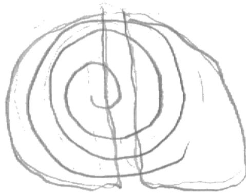
A cyclotron is a type of particle accelerator. Charged particles move inside the cyclotron in a circular motion with a centripetal force. In a cyclotron two hollow electrodes are used, the charged particles ~~generate~~ travel in a circular motion from one electrode to the other crossing a gap. This movement across the gap creates a potential difference.
