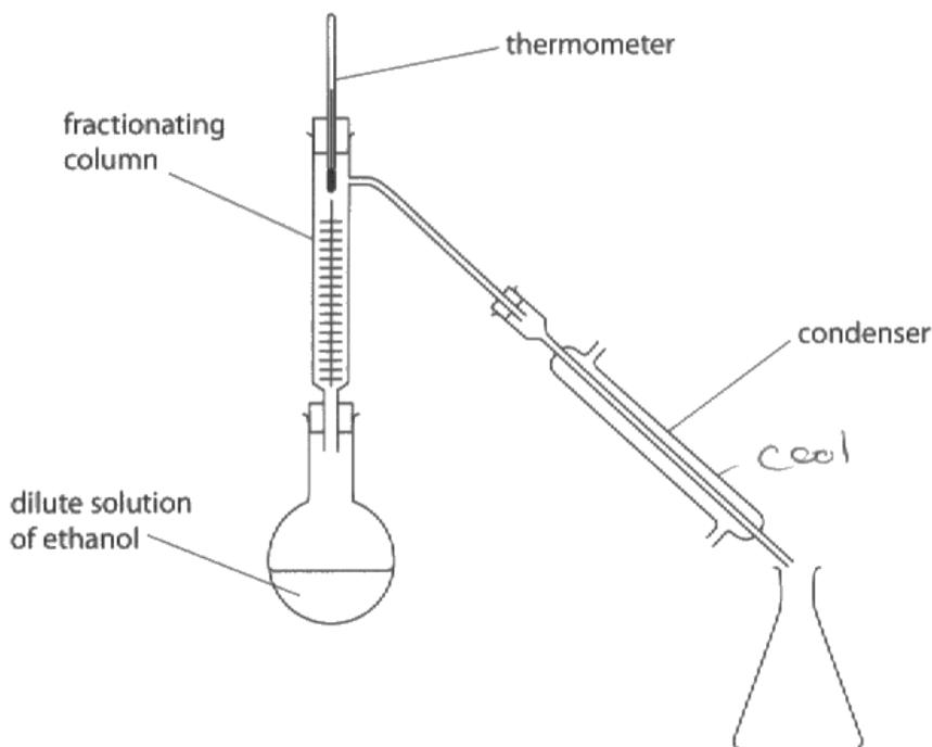
Describe how this apparatus is used to obtain a more concentrated solution of ethanol.
