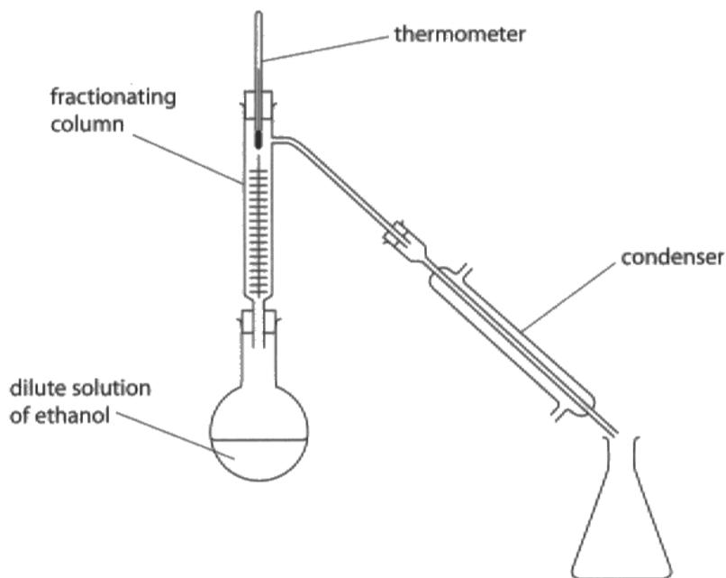
Describe how this apparatus is used to obtain a more concentrated solution of ethanol.
