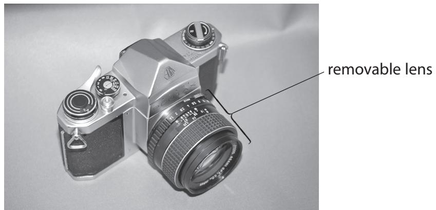
One of the pieces of glass is radioactive. Its surface is covered with a thin layer of magnesium fluoride.
