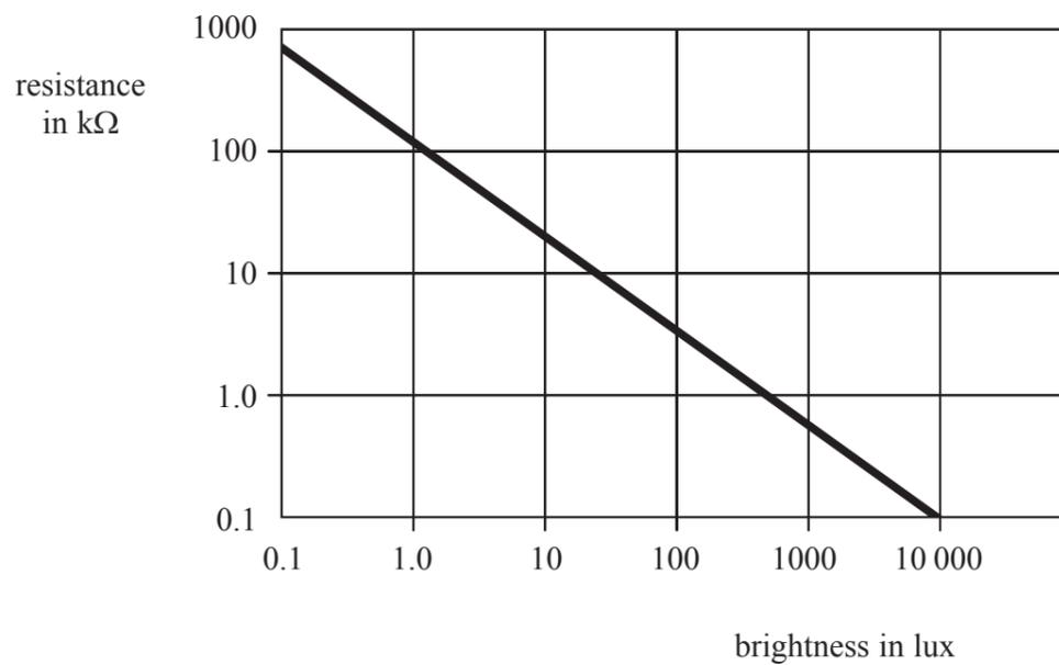
There is a current of 0.02 mA in the light-dependent resistor when the voltage across it is 2 V.
