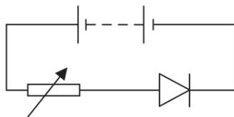
There **is no current** in the circuit when the battery is reversed.
