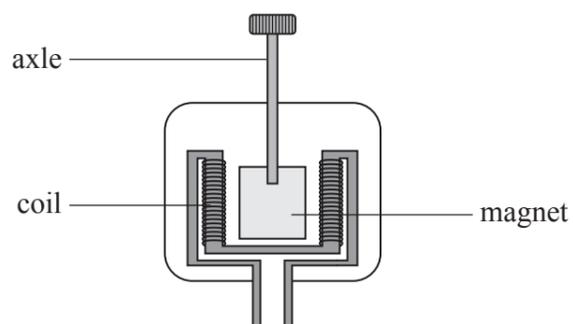
In the dynamo, which of these will increase the size of the voltage generated?
